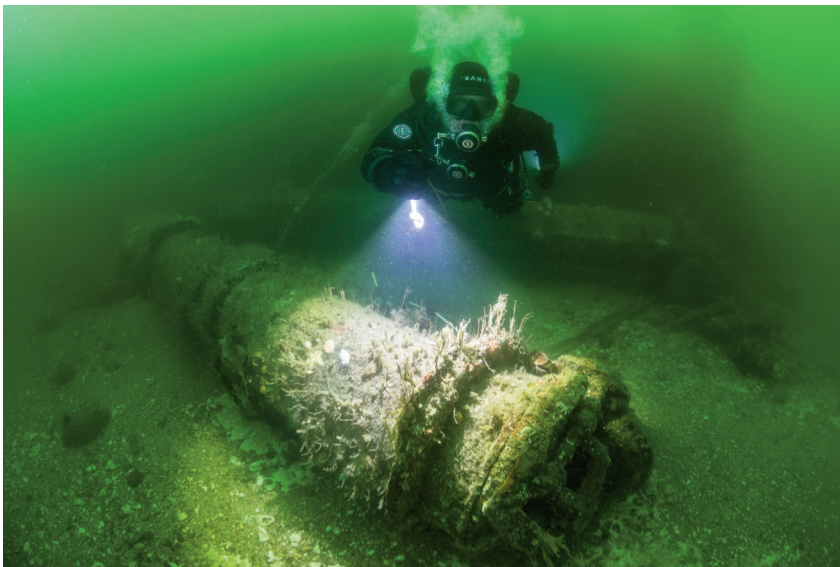
Fig. 17: UC 71, diver next to the torpedoes, which have fallen off between 2016 and 2019, a further foreboding sign that UC 71 is slowly decaying (F. Huber)
