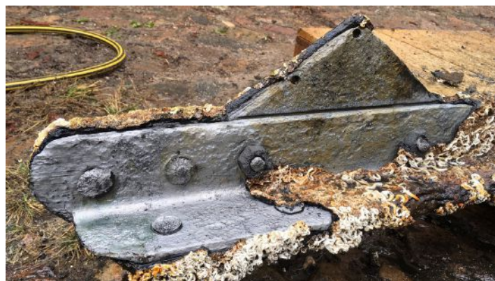
FIGURE 3. The net cutter is astonishingly well-preserved. After the initial rough cleaning, the original gray coat of paint began to show through the layer of corrosion. (Photo courtesy of Florian Huber.)
